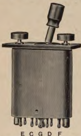
FIG. 120.—Cook Listening and Ringing Key. A hard rubber partition runs in the length of the case, so that it divides the instrument into two equal parts; one E , one C , one G , etc., being on either side, making double connections, as shown.
